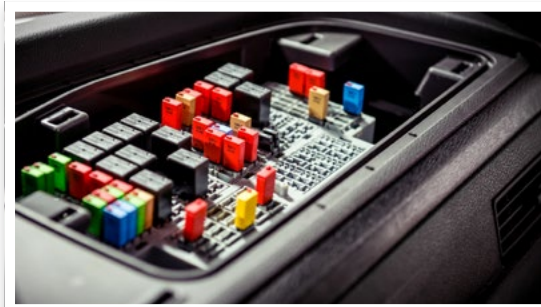
In-cab electrical panel
